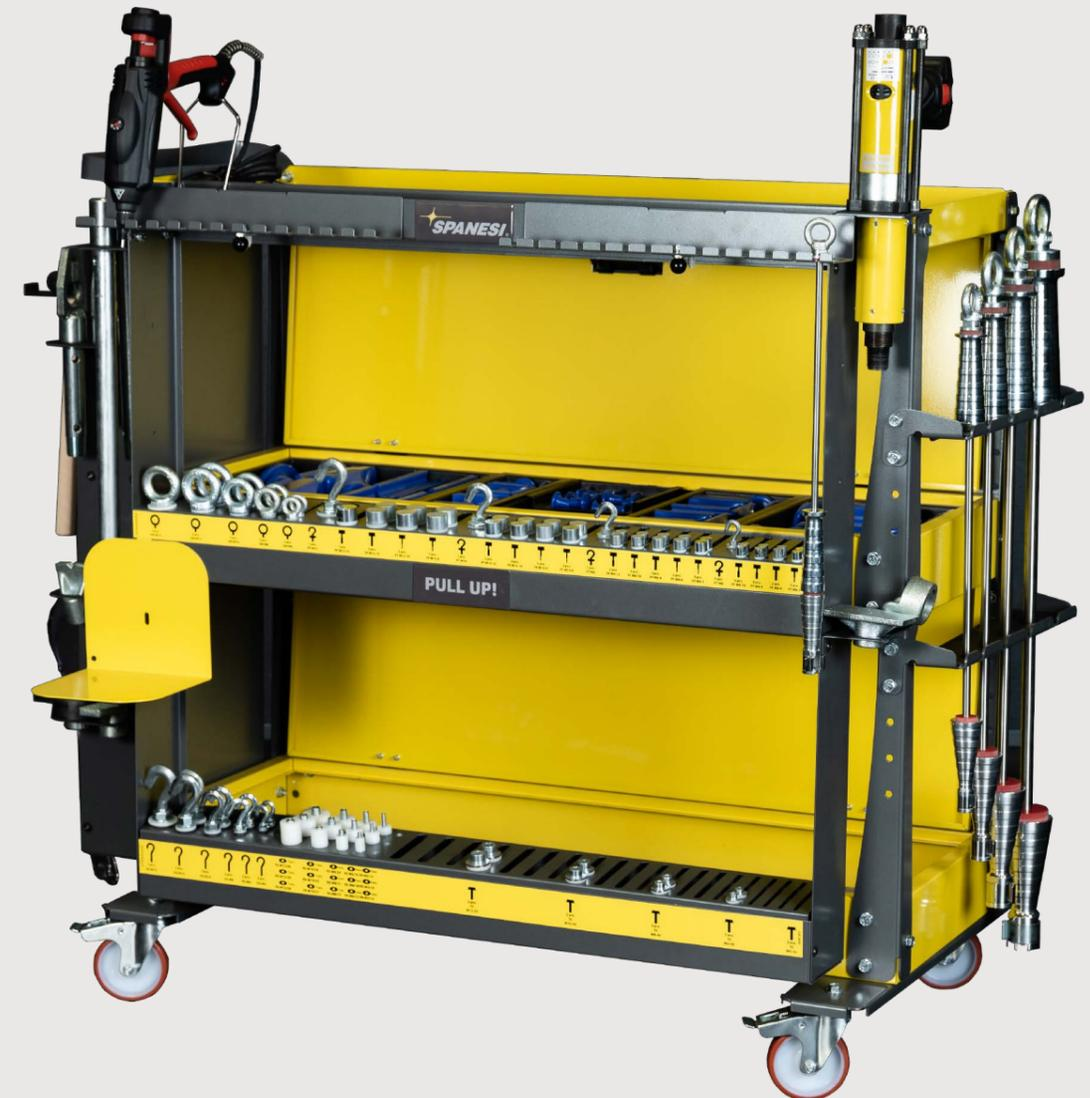
The repair solution for small to moderate damage types. Up to 2 suction cups may be combined for simultaneous pulls. Can be used with the Electro puller system (optional).
